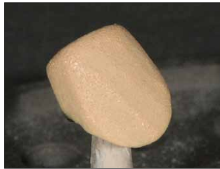
By simply applying the orange-coloured Base Opaque superb bonding to the PFM alloy is achieved.
